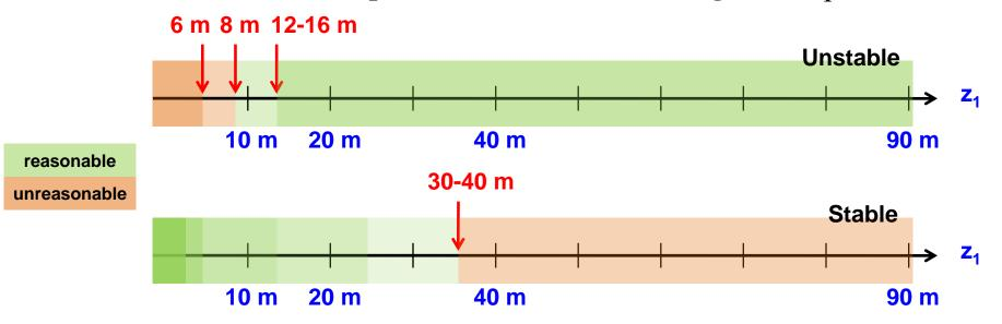
: The lowest model layer height about **10 m** is suggested as **an optimal value** that can be **satisfactory for both unstable/stable conditions**.
